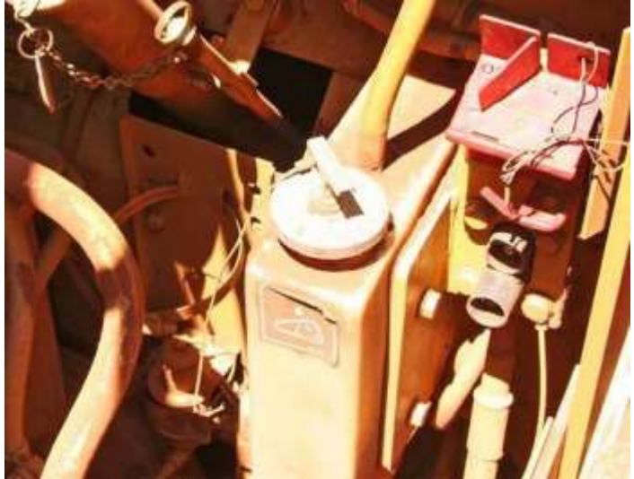
Pivot Shaft Oil Reservoir
