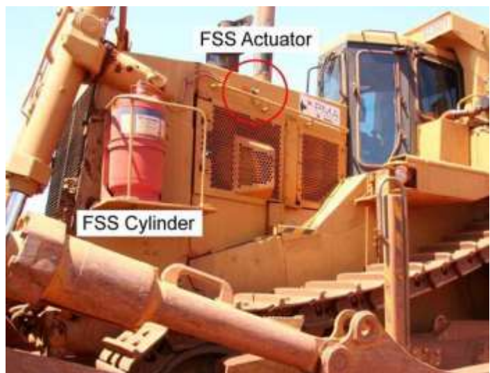
Fire Suppression System
